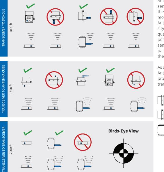
Antenna positions for the sending Transceiver and the corresponding receiving Dongle, Fixture Antenna or Transceiver can significantly affect signal quality. For optimum performance reference the sending and receiving pairings and positions in the diagrams to the left.
