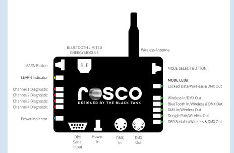
The CubeConnect system was designed for applications which can not support expensive 3rd party full-speed wireless DMX hardware, but require dynamic or static effects. The patented CubeConnect algorithm automatically compresses the incoming DMX data to maximize throughput to the dongles by only sending DMX channels which changed from the previous frame.
